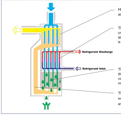
Maximum heat transfer is achieved in the air-to-air heat exchangers cross-flow design
