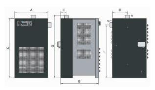
Please note; inlet air connection is located on top of unit for models ACT12-ACT1000. Dimensions include connection fitting. Dimensions are rounded to the nearest inch.
